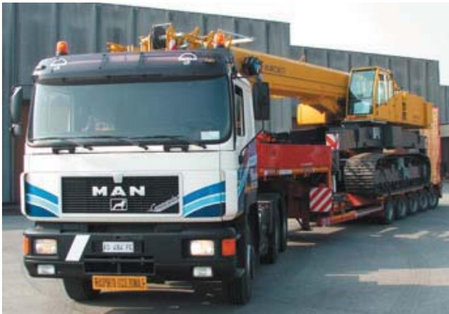
The **SHERPA** is a very compact crane and it is hauled without removing ANYTHING. Crawlers and counterweight remain fitted to the machine.
