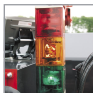
Overload warning lamps + auto stop + alarm
